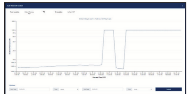
CableGuardian portal showing IR readings for the Sub-Network Section.
